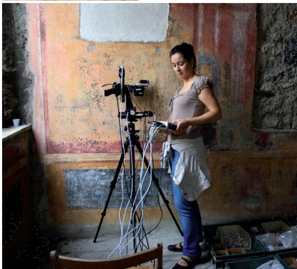
Fig. 5. Anastasia Giakoumaki performing micro-Raman measurements on the originally red side field in triclinium (16). It had to be done in the absence of wind in order to avoid vibrations in the tripod.
