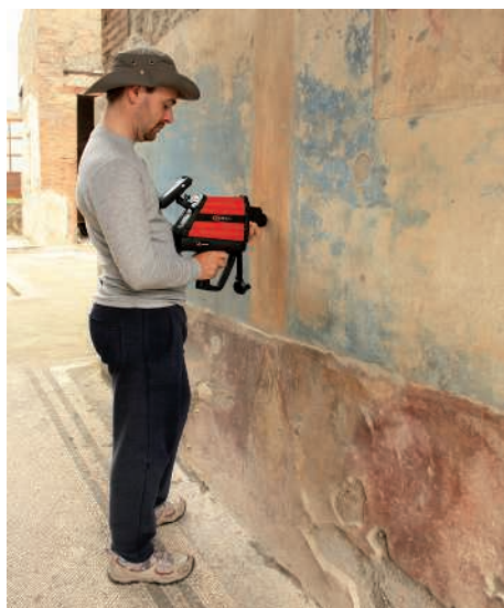
Fig. 4. Kepa Castro with the DRIFT instrument, measuring wall painting remains of the right (south) wall in fauces (1).
