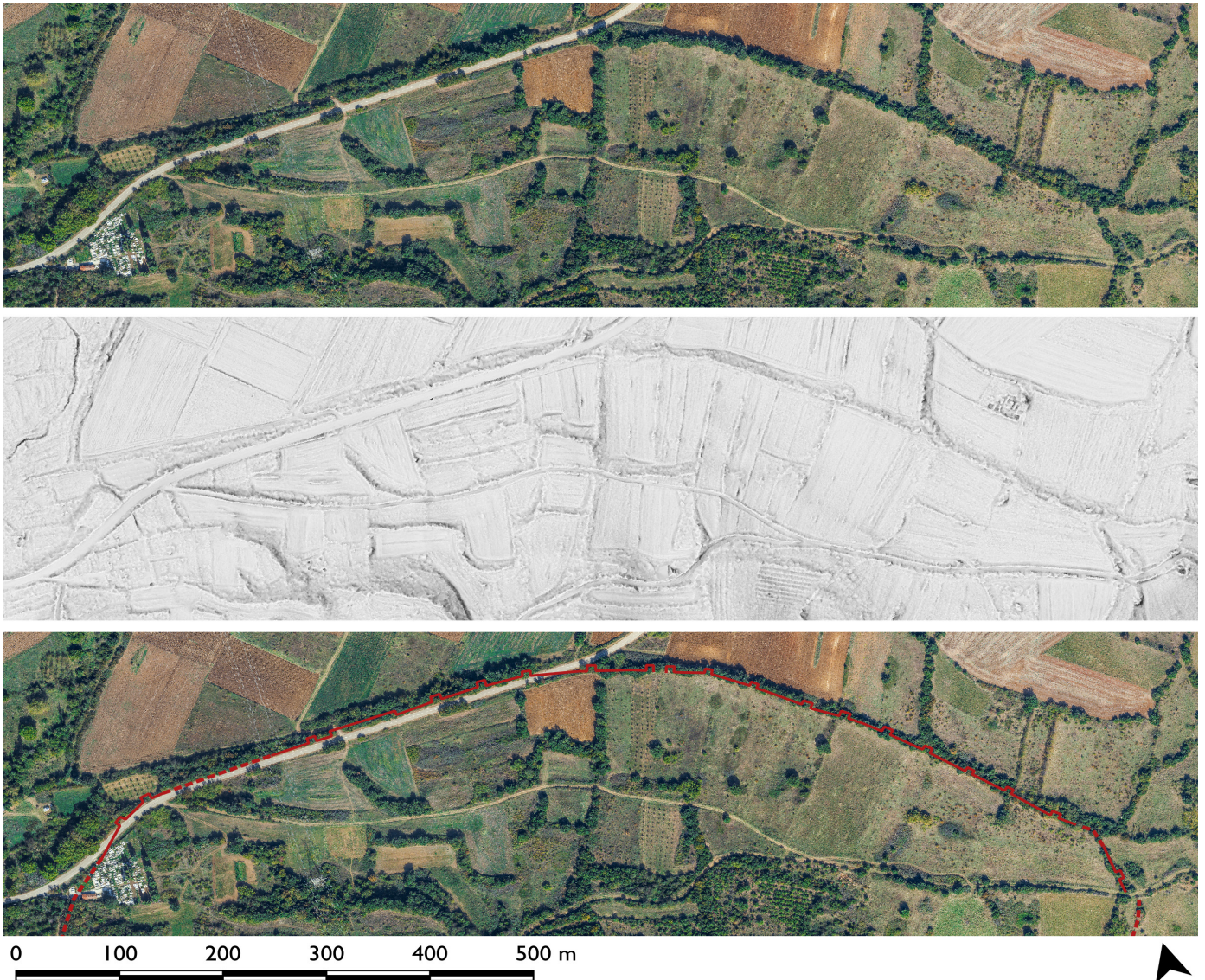
Fig. 21: Kato polis fortifications at Melitaia. Top: Aerial orthographic photomosaic of fortification line area. Middle: DTM-derived topographical relief model of same area. Bottom: Aerial photograph with superimposed and rectified drawing of fortifications derived from Lolling ( Lolling 3 ) and DTM. Plans by the author.
